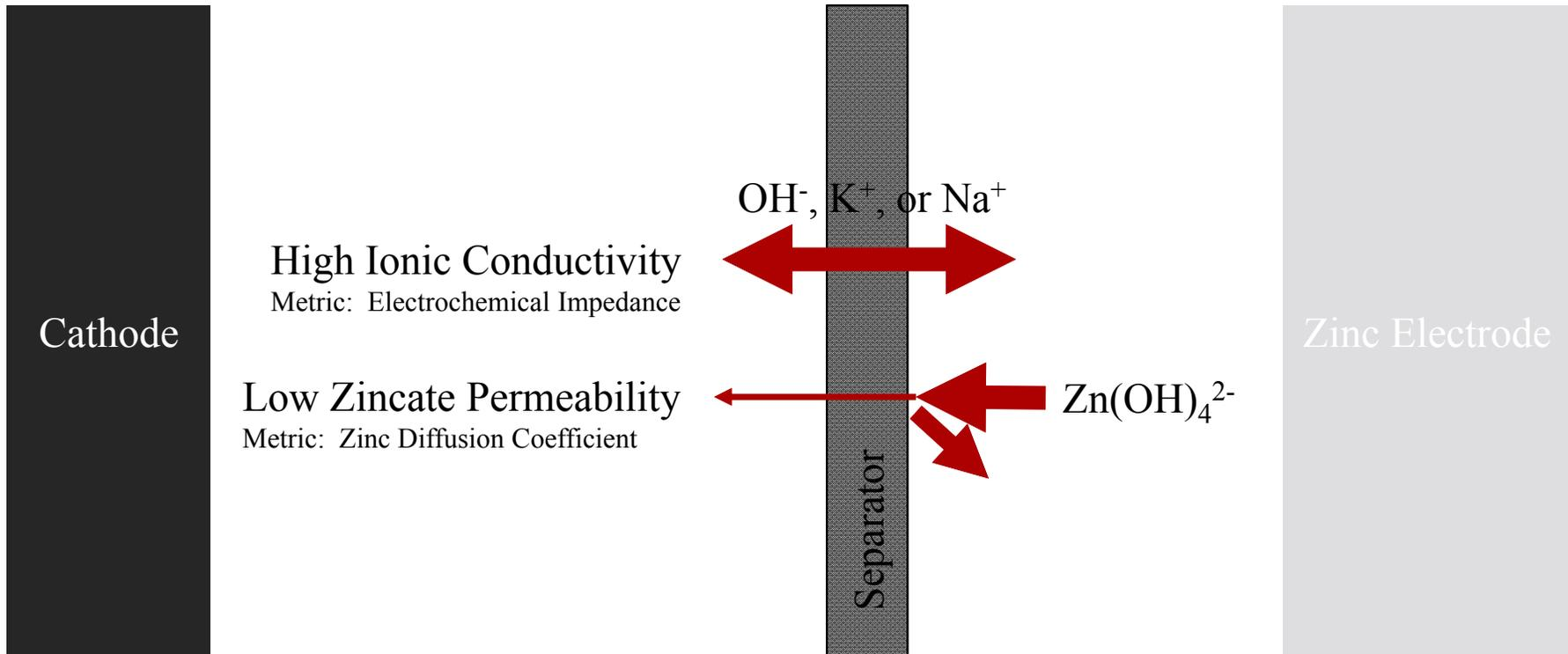
*A selective membrane/separator is needed that allows charge carrying ions through but blocks or limits Zn (zincate)*
